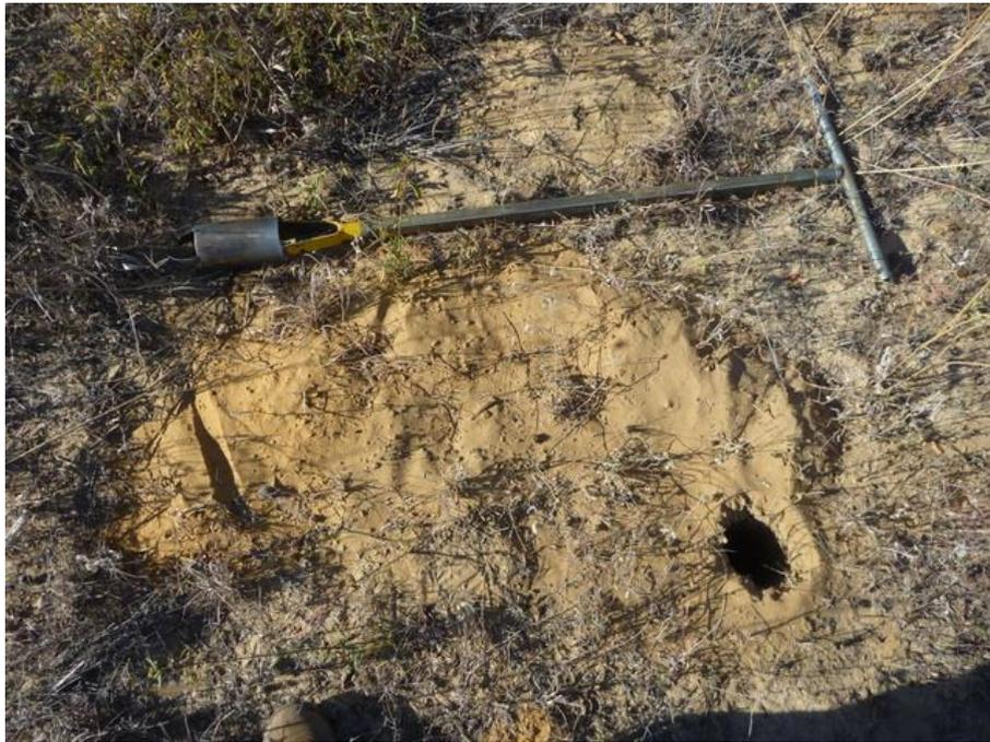
**Figure 15: Auger profile of a deep sandy Fernwood with a degree of yellowing in the subsoil**
