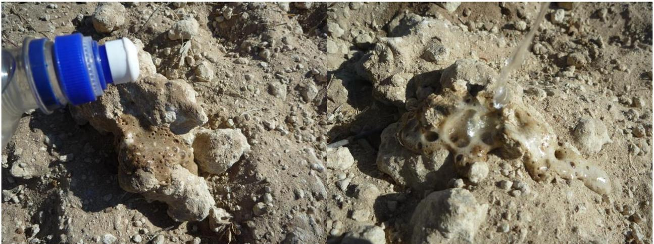
**Figure 16: Addition of HCl (10 % solution) to subsoil lime (left) and effervescence confirming the presence of carbonates (right)**
