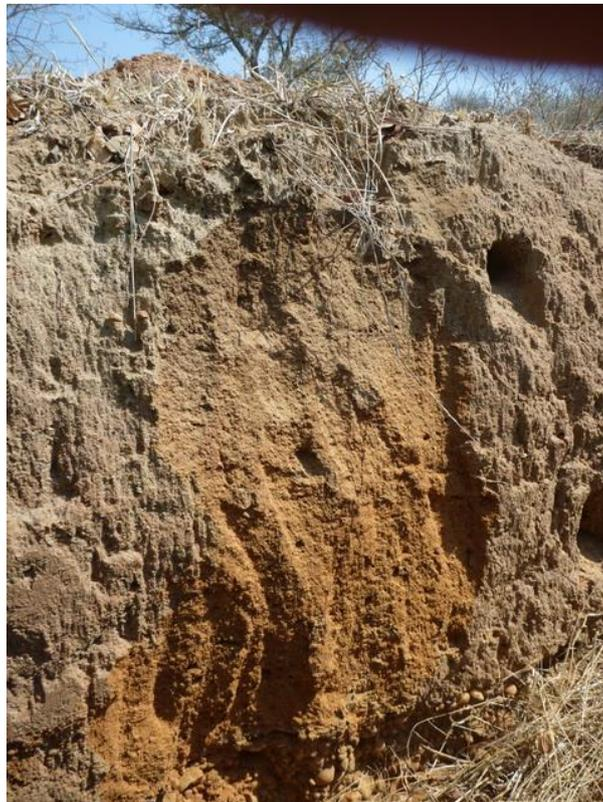
**Figure 8: Exposed profile of the Clovelly soil form in site Alternative 1**
